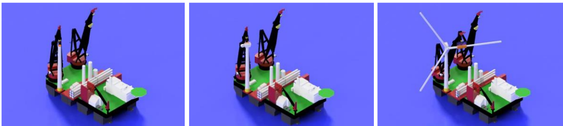
Figure 13: Assembly of tower section, assembly of nacelle on tower section, blade installation, delivered for the SBOS project by HES.
