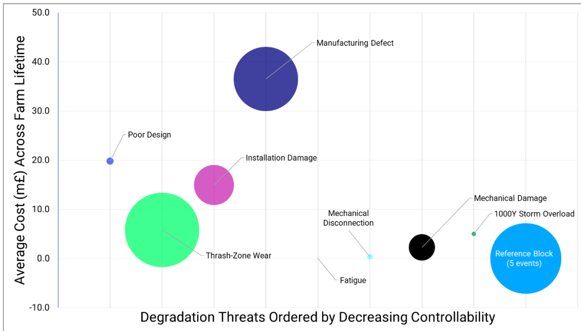
Figure 17: Cost and occurrence of degradation threats across a 50-unit farm.
