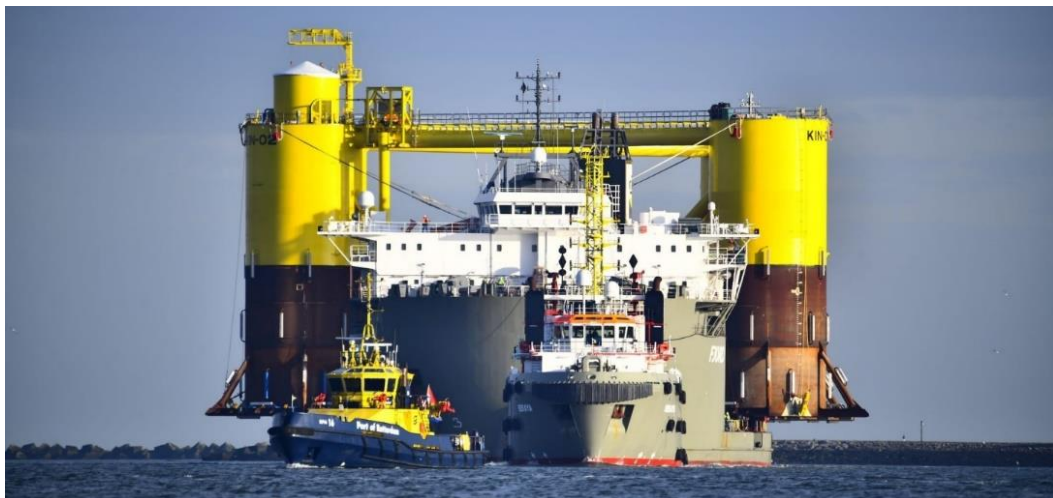
Figure 4: Kincardine semi-submersible foundation transport overhand, courtesy of Boskalis.
