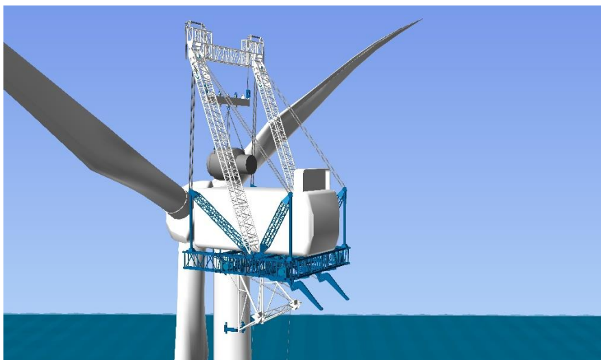
Picture 2 Nacelle modular lift device
