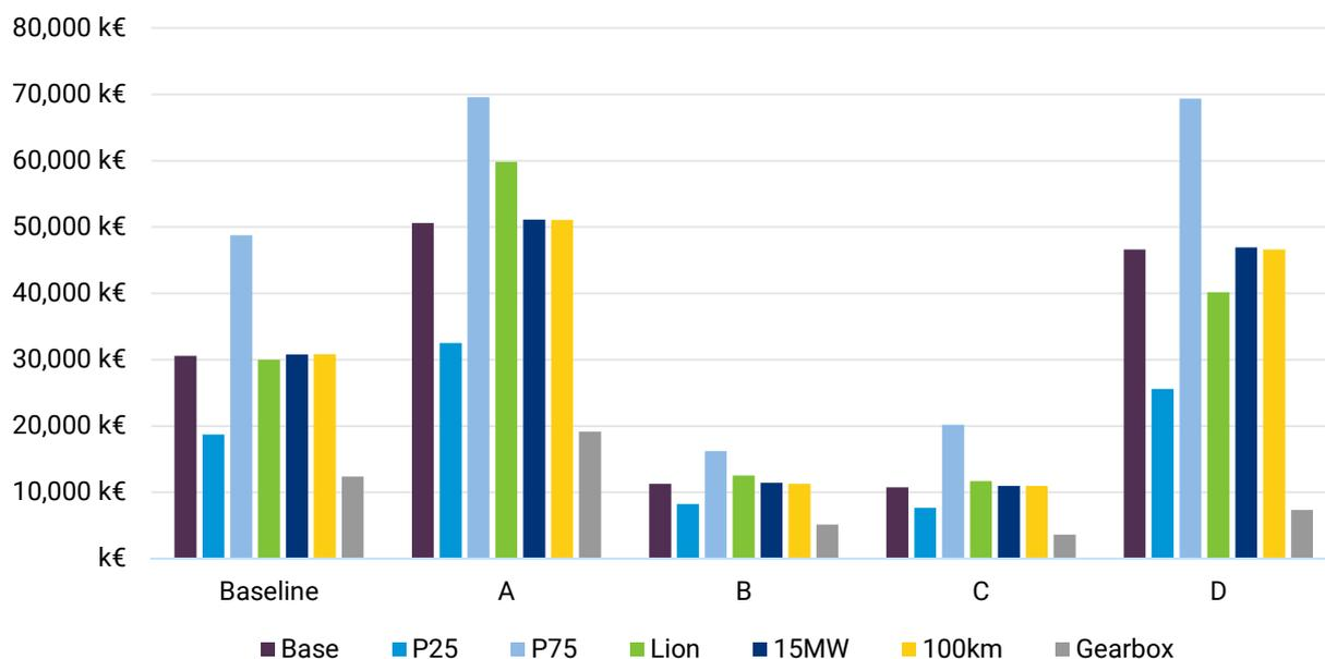
**Figure 7: HLM campaign exchange costs. Base refers to the 10MW blade set exchange at Hywind Scotland conditions, 50km to port with P50 conditions scenario.**
