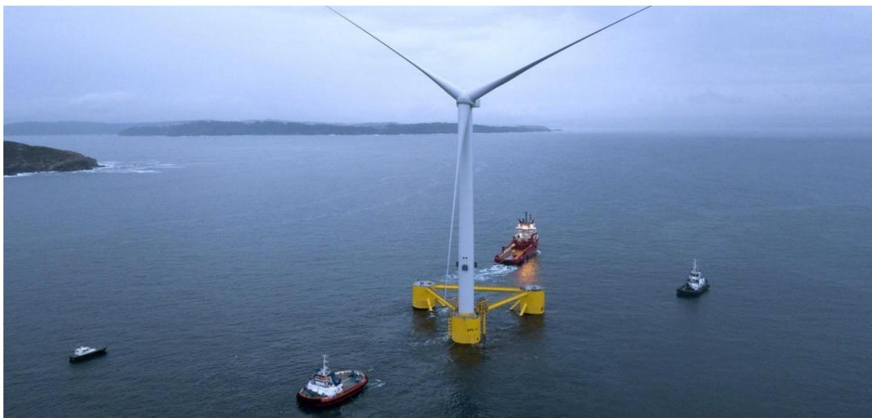
**Figure 9: WindFloat Atlantic tow from port to site operation**
