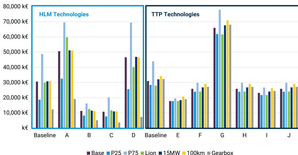
**Figure 12: Comparison of HLM & TTP campaign exchange costs. Base refers to the 10MW blade set exchange at Hywind Scotland conditions, 50km to port with P50 WoW conditions scenario.**
