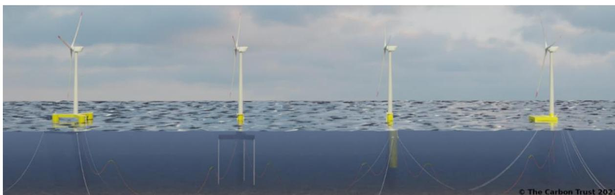
**Figure 13: Typical floating offshore wind substructures and mooring configurations (from left to right: semi-submersible, tension leg platform (TLP), spar and barge platforms)**
