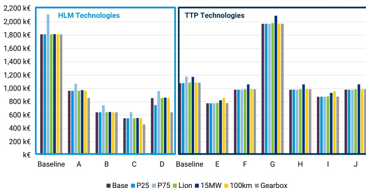
**Figure 11: Comparison of HLM and TTP single exchange costs. Base refers to the 10MW blade set exchange at Hywind Scotland conditions, 50km to port with P50 WoW conditions scenario.**
