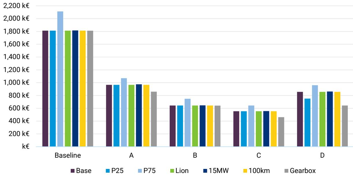
**Figure 8: HLM single component exchange costs. Base refers to the 10MW blade set exchange at Hywind Scotland conditions, 50km to port with P50 conditions scenario.**
