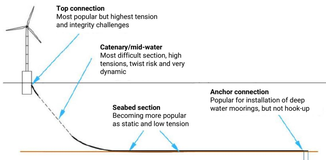
Figure 15: Typical hook-up locations (Courtesy of First Energy Development)
