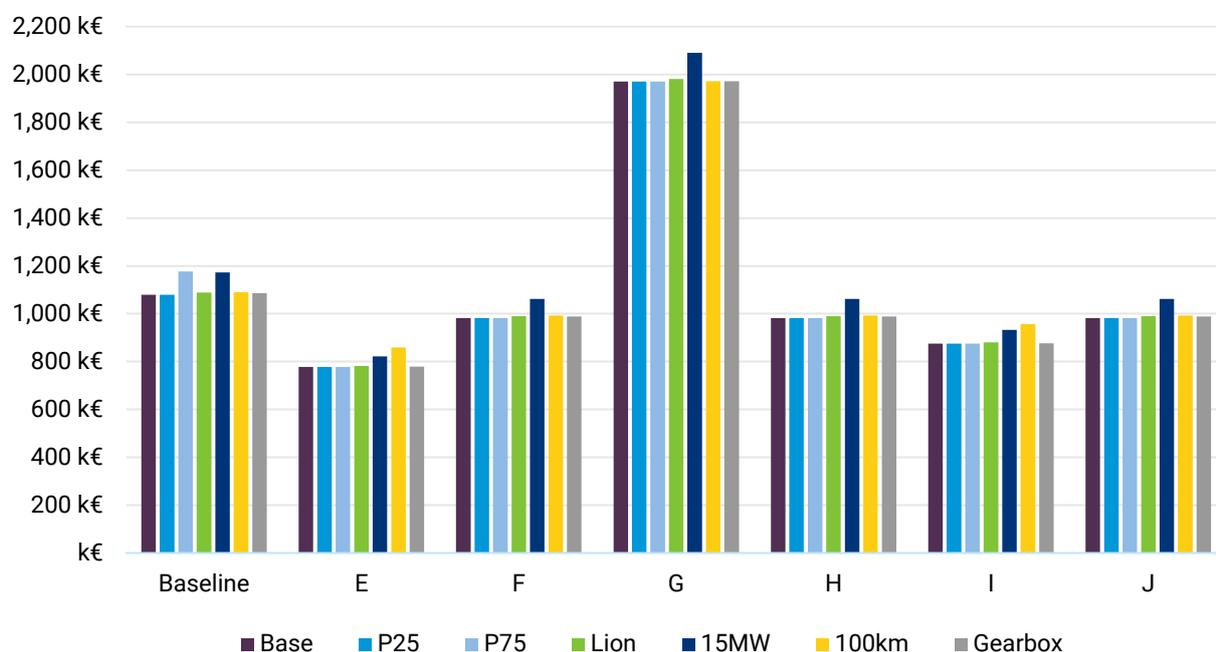
Figure 10: TTP Single component exchange costs. Base refers to the 10MW blade set exchange at Hywind Scotland conditions, 50km to port with P50 WoW conditions scenario.
