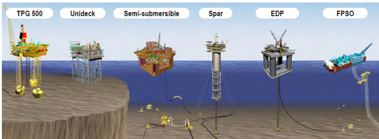
Figure 2.3.1. Floating structures used in the oil and gas industry (Maine University, 2010)
