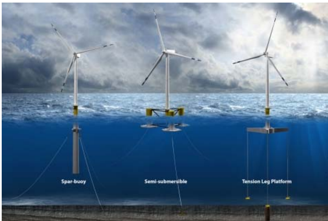
Figure 2.1.1. Floating wind foundation typologies (DNV-GL, 2014)
