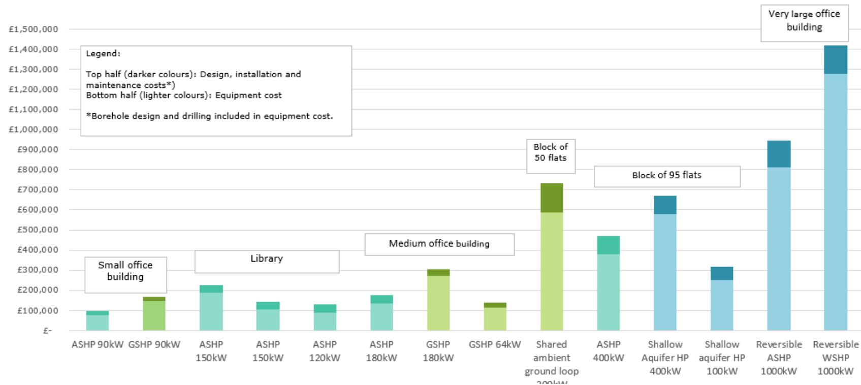
Figure 37: Upfront capital costs: medium to large scale heat pumps in communal heating and non-domestic building (not including heat emitters or distribution)
