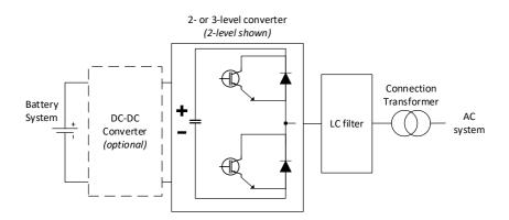
Figure 1: Simplified schematic of a 2- or 3-level converter with battery in the DC link
