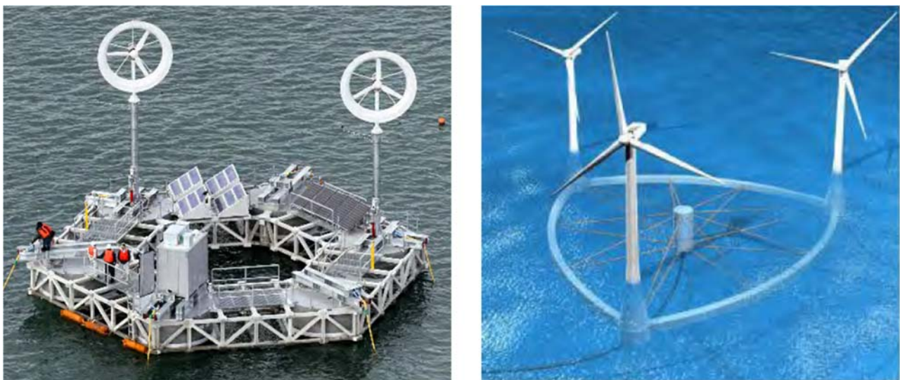
Figure 68. WindLens (L) and Shimizu (R) semi-submersible designs (Maine International Consulting, 2013).
