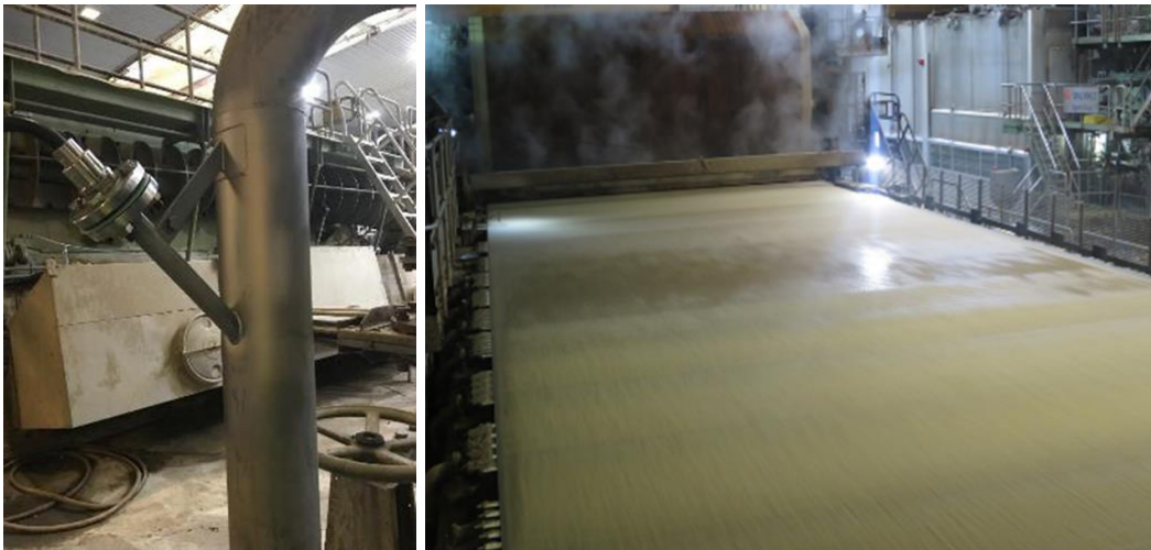
Figure 4 FBRM probe installed in the approach flow to PM4 (L). Progressive removal of water from the paper web by gravity and vacuum suction on the wire section of PM4 (R)
