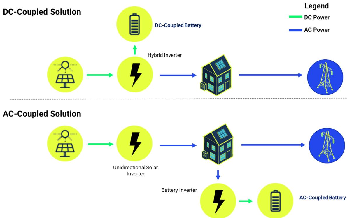
*Figure 2: Comparison between DC-Coupled (Top) and AC-Coupled (Bottom) Solutions*
