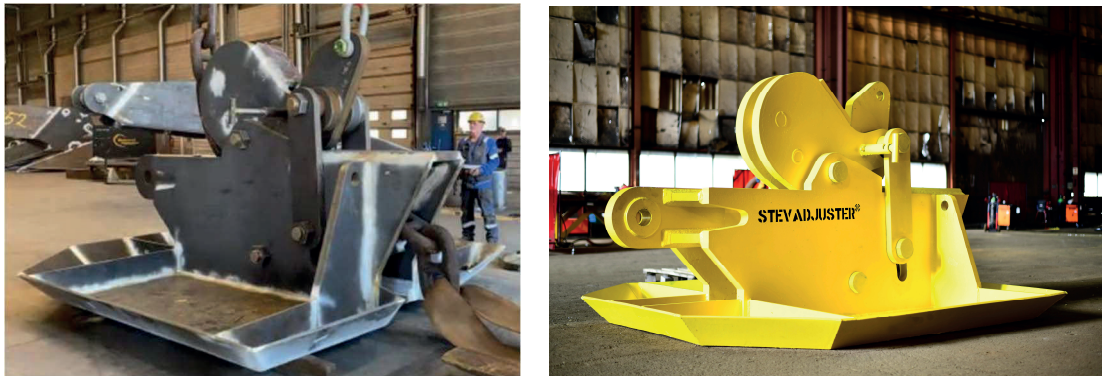
Stevadjuster® factory testing & painting ready for delivery
