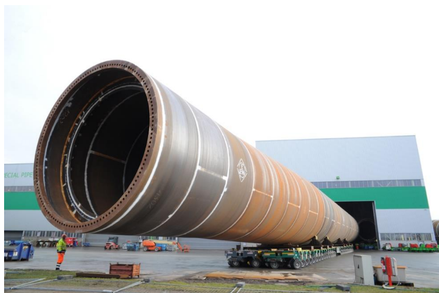
Figure 39. XXL monopile fabrication (EEW, 2016)
