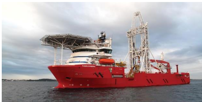
Figure 38: Typical fit-for-purpose vessel used for geotechnical and geophysical surveys in offshore wind (Fugro)
