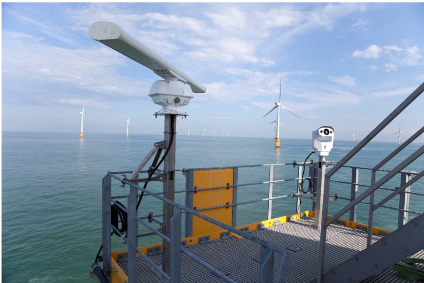
Figure 23. TADS Camera-radar unit installed in Thanet.
