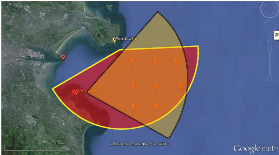
Figure 13: Illustration of PPI scan arcs for Windcube 400S devices
